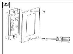
Attach front cover to wall control with screws provided.
